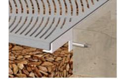
For retrofit application in saw cut concrete. Use (leg down orientation) when existing hole is same as grate size.
